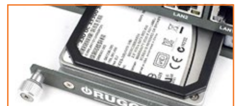
MILCORTEX 1300 features 1 front-loading 2.5" SSD bays with convenient thumbscrew fasteners
