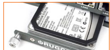
MILCORTEX 2100 features 2 front-loading 2.5" SSD bays with convenient thumbscrew fasteners
